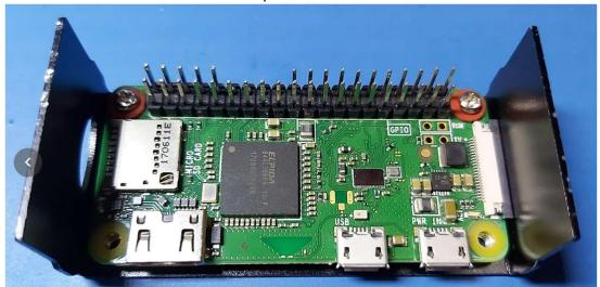
4. Install the MMDVM Board by plugging it into the Raspberry Pi. Note that the pins from the OLED are not touching any of the pins on the Raspberry Pi.
