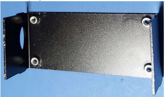
3. Install the Raspberry Pi into the lower case using the 2 short screws next to the header pins. Note the SD Card Slot is on the left in the photo.
