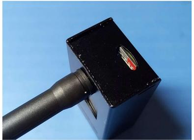
7. Screw on the antenna. Don't install the SD Card Yet as we need to install the software onto it.
