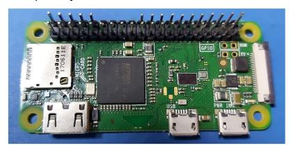
There are two versions of the Raspberry Pi Zero W and Raspberry Pi Zero WH. The "W" version does not come with headers and the "WH" version includes headers pre-soldered.
