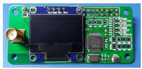
This board provides the RF interface between the Raspberry Pi and your DMR radio.
