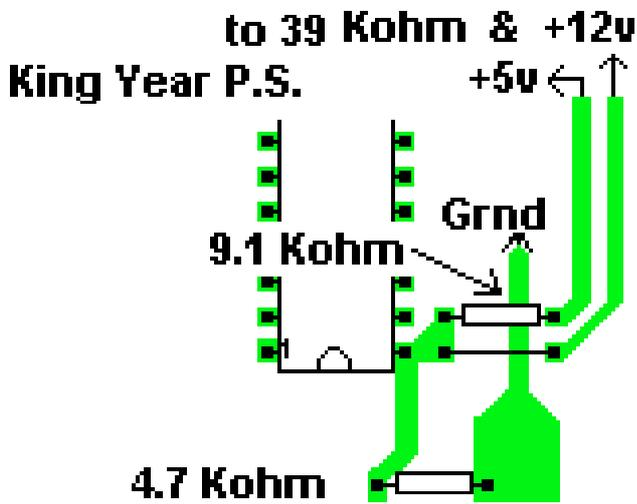
You should find a resistor from pin 1 to ground. In most instances this resistor is a 4.7 Kohm. There should be another resistor from pin 1 to the +5 volt track. This resistor could be a 9.1 Kohm if there is another resistor from pin 1 to the +12 volt track. This resistor could be a 39 Kohm resistor. Above is the circuit for pin 1 of a King year power board. The 39K-ohm resistor is where the +12volt supply main feed is located on the other end of the board.
