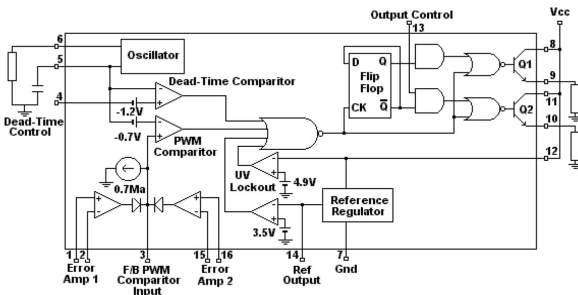
Pin 6 is earthed through a suitable resistor and pin 5 is connected through a suitable capacitor to earth.
