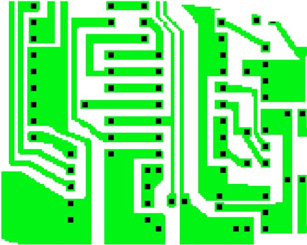
The above diagram is portion of the component side of a typical board. Note pin 1 of the I.C. This is the underside of the same section. Can you identify the pins of the I.C.
