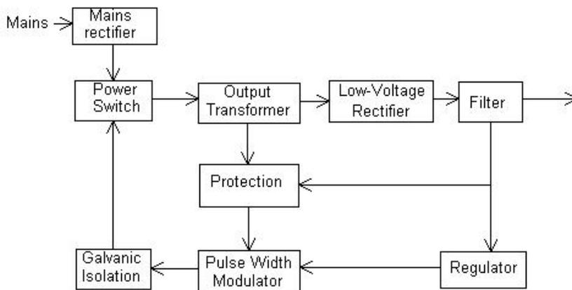
Fig 1: Block Diagram of a power supply with primary switching.
